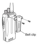
If necessary, attach the belt clip using the two supplied M3 x 8 mm screws.
